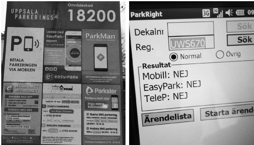
Figure 12.4. Ticket machine illustrating multiple payment solutions for parking (left) and a snap shot showing the user interface of the handheld device for the ticket control staff (right). Pictures from (Markendahl & Laya, 2013). Photo: Jan Markendahl.
